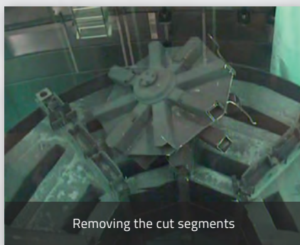
Segmentations of "hot components" inside the cooling pond of the nuclear power plant
